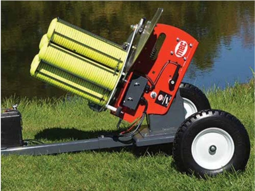
The 200E Sporter is the entry level club sporting clay target machine made in the USA. The tilt base upgrade can be added at any time, turning a good machine into a great machine! It holds 200 standard targets and has a genuine 90 yard throwing distance. Machine elevates back to 70 degrees and has a three-year warranty, as well as a life-time warranty on the main-shaft and one-way bearing.
